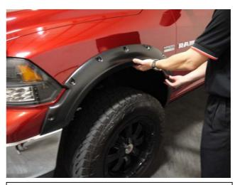
**STEP 8:** Place the Fender Flare onto the vehicle and fit into the correct position following the contours of the body.
