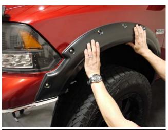
**STEP 10:** Check fitment and contour of Fender Flare to headlight housing and readjust if necessary.
