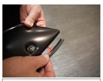
**STEP 12:** Attach the included rubber seal to the Fender Flares. Peel back 2" of the adhesive backing and position on the Fender Flare. Attach the seal to the fender flare, peeling back a few inches at a time. Attach rubber seal along all areas the Fender Flare will make contact with the vehicle body. Trim any excess rubber seal.
