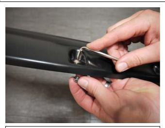
**STEP 1:** Attach 9 bolts to each Fender Flare using a 3/16" Allen key and a 10.0mm wrench/socket. (wrench/socket and Allen key not supplied). Ensure inside of Fender Flares where the rubber seal is attached is clean, using the alcohol wipes provided. Wipe away any residue with a dry clean cloth. For Ram 2500 and 3500, only 8 bolts are used.
