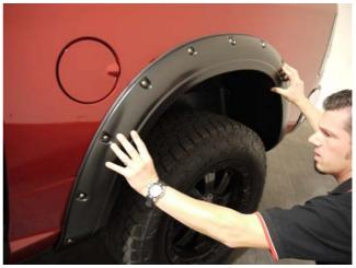
**STEP 14:** Remove all factory bolts and retain for installation of Fender Flares.
