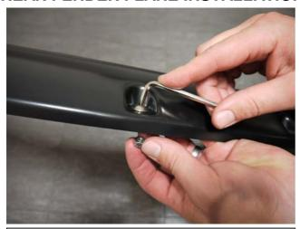
**STEP 11:** Attach 11 bolts to each Fender Flare using a 3/16" Allen key and a 10.0mm wrench/socket. (wrench/socket and Allen key not supplied) Ensure inside of Fender Flares where the rubber seal is attached is clean, using the alcohol wipes provided. Wipe away any residue with a dry clean cloth.
