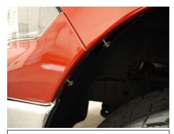
**STEP 7:** Remove all factory bolts and retain for installation of Fender Flares.
