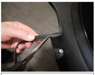
**STEP 4:** Cut notches in extrusion tape to allow it to fit neatly around headlamp area of flare as shown.
