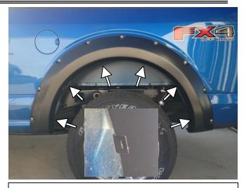
**STEP 16:** Place the Fender Flare onto the vehicle and fit into the correct position following the contours of the body. Use 6 of the U-style clips to secure the Fender Flare to the body. Make sure the barb in the clip securely attaches in the slot on the Fender Flare.
