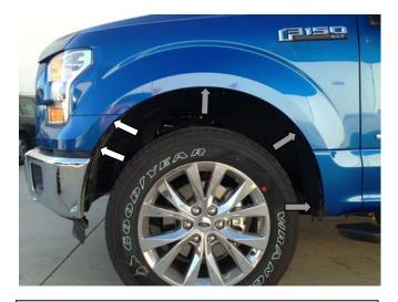
**STEP 6:** Locate three (3) 5.5mm bolts and two (2) 7mm bolt.
