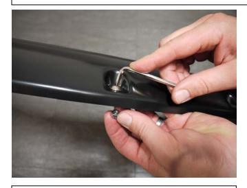
**STEP 1:** Attach 9 bolts to each Fender Flare using a 3/16" Allen key and a 10.0mm socket wrench/socket. (wrench/socket and Allen key not supplied) Ensure inside of Fender Flares where the rubber seal is attached is clean, using the alcohol wipes provided. Wipe away any residue with a dry clean cloth.
