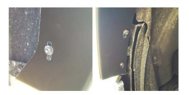
**STEP 9:** Reinstall the remaining 5.5mm bolt and two 7mm bolts.
