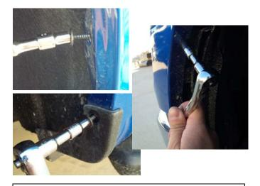
**STEP 7:** Remove three (3) 5.5mm bolts and two (2) 7mm bolt, retain for installation of Fender Flares.
