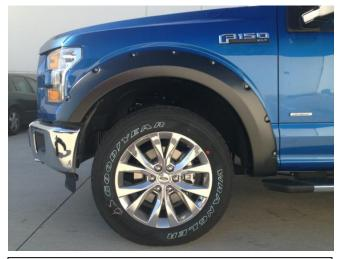
**STEP 10:** Repeat installation method for other side. Double check the front Fender Flares to make sure all bolts are tight and clips are securely fastened.
