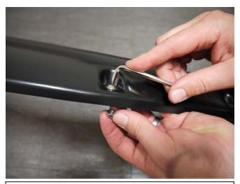
**STEP 11:** Attach 9 bolts to each Fender Flare using a 3/16" Allen key and a 10.0mm socket wrench/socket. (wrench/socket and Allen key not supplied) Ensure inside of Fender Flares where the rubber seal is attached is clean, using the alcohol wipes provided. Wipe away any residue with a dry clean cloth.
