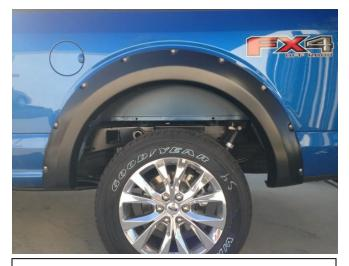
**STEP 17:** Repeat installation method for other side. Double check the front Fender Flares to make sure all bolts are tight and clips are securely fastened. Your installation is now complete. Do not use abrasive cleaners.
