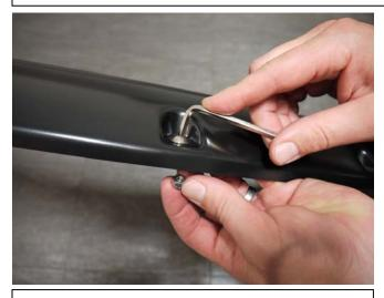
**STEP 1:** Attach 9 bolts to each Fender Flare using a 3/16" Allen key and a 10.0mm socket. (wrench/socket and Allen key not supplied) Ensure inside of Fender Flares where the rubber seal is attached is clean, using the alcohol wipes provided. Wipe away any residue with a dry clean cloth.
