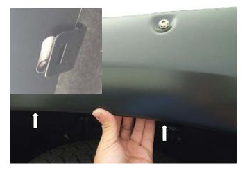
**STEP 7:** Place the Fender Flare onto the vehicle and fit into the correct position following the contours of the body. Locate the 2 mounting slots on the top of the fender flare. Use 2 of the large U-style clips (indicated with an X on the clip) to attach the fender flare to wheel arch. Make sure the barb in the clip securely attaches in the slot on the Fender Flare.
