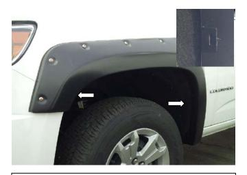
**STEP 8:** Use 2 of the small U-style clips to secure the Fender Flare to the body. Make sure the barb in the clip securely attaches in the slot on the Fender Flare.
