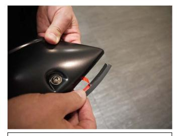
**STEP 12:** Attach the included rubber seal to the Fender Flares. Peel back 2" of the adhesive backing and position on the Fender Flare. Attach the seal to the Fender Flare, peeling back a few inches at a time. Attach rubber seal along all areas the Fender Flare will make contact with the vehicle body.
