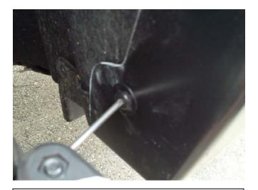
STEP 9: Reinstall the #15 Torx head screw.
