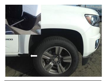
**STEP 6:** Locate the Torx screw at the lower section of the wheel well. Remove the Torx screw using a #15 Torx head screwdriver. Retain the screw for installation.
