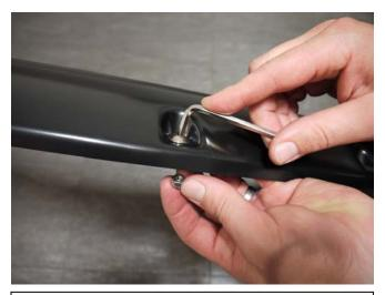
**STEP 11:** Attach 9 bolts to each Fender Flare using a 3/16" Allen key and a 10.0mm. (wrench/socket and Allen key not supplied) Ensure inside of Fender Flares where the rubber seal is attached is clean, using the alcohol wipes provided. Wipe away any residue with a dry clean cloth.
