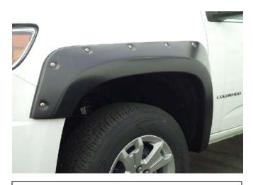
**STEP 10:** Repeat installation method for other side. Double check the front Fender Flares to make sure all bolts are tight and clips are securely fastened.
