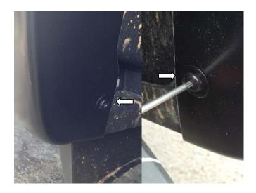
STEP 18: Reinstall the #15Torx head screws.
