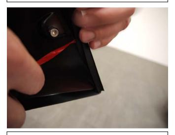
**STEP 13:** Pulling at right angles to the extrusion, remove the liner from the extrusion in small portions and apply thumb pressure to ensure that it adheres to the Fender Flares.
