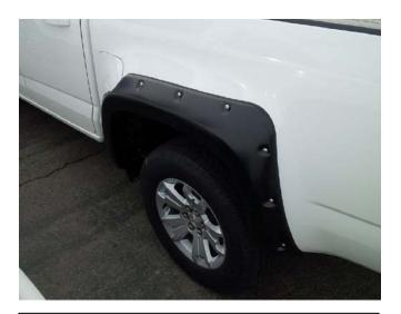
**STEP 19:** Repeat installation method for other side. Double check the front Fender Flares to make sure all bolts are tight and clips are securely fastened. Your installation is now complete. Do not use abrasive cleaners.
