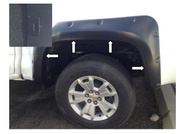
**STEP 17:** Place the Fender Flare onto the vehicle and fit into the correct position following the contours of the body. Use 4 of the U-style clips to secure the Fender Flare to the body. Make sure the barb in the clip securely attaches in the slot on the Fender Flare.
