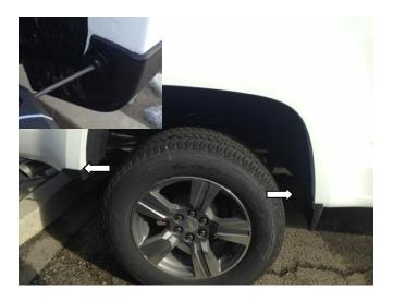
**STEP 16:** Locate the 2 outer screws. Remove the screws using a #15 Torx head screwdriver. Retain screws for installation.
