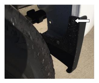
**STEP 13:** Using #15 Torx head screwdriver remove upper screw from the front factory mud guard in the rear wheel arch. Maintain screws for re-install.
