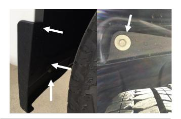
**STEP 5:** For models <u>WITH FRONT</u> factory mud guards, remove using #15 Torx head screwdriver at the upper and lower screw locations from the front factory mudguards and M10 socket at the underside location indicated above, maintain #15 Torx head screws for re-install. Retain factory mudguards for later use if required, Fender Flares require the mud guards to be removed.
