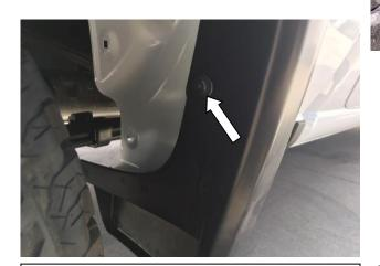
**STEP 16:** Using #15 Torx head screwdriver reinstall the upper screw from the front factory mud guard in the rear wheel arch through the slot in the Fender Flare.
