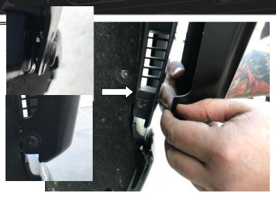
**STEP 7:** Place Fender Flare on the vehicle into the position of best fit. Peel back 2 inches of the red tape liner on the double-sided tape of the fender flare extrusion at both ends, ensure liner is on the outside of part ref to step 9
