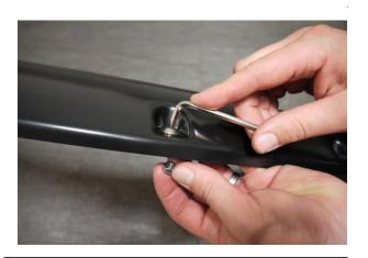
**STEP 10:** Attach the bolts and nuts to each Fender Flare using 3/16" Allen Key/Torx and a 1/2" wrench/socket (wrench/socket and Allen key not supplied). Ensure inside of Fender Flares where the rubber extrusion is attached is clean, using the alcohol wipes provided. Wipe away any residue with a dry clean cloth.
