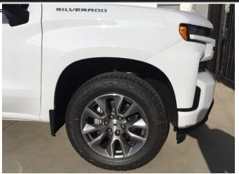
**STEP 4:** Clean the body areas where the Fender Flares will make contact. Ensure fenders are dry prior to install. Turn tires outward for Fender Flare installation.
