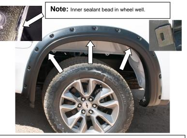
**STEP 17:** To secure the Fender Flare to the body, apply upward tension on Fender Flare to the vehicle fender when installing the black metal clips. Slide the clips over the Fender Flare and the inner wheel arch lip in the three locations shown. Position the clip so that the barb in the clip locates in the slot of the Fender Flare. Ensure all mounting points are tight and secure and that the extrusion is flush neatly against the vehicle body. Repeat install steps for the opposite side.
