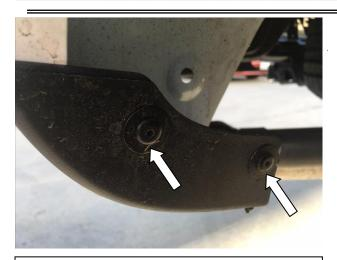
**STEP 14:** Using #15 Torx head screwdriver remove the two bottom screws from the rear factory mud guard. Maintain screws for re-install.
