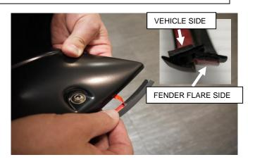
STEP 2: NOTE: FRONT FENDER FLARES REQUIRE EXTRUSION WITH (2) DOUBLE SIDED TAPES. Attach the included rubber extrusion to the Fender Flares. Peel back 2" of the adhesive backing and position on the Fender Flare. Attach the extrusion to the Fender Flare, peeling back a few inches at a time. Ensure pressure is used to secure rubber extrusion to Fender Flare edge. Attach rubber extrusion along all areas the Fender Flare will make contact with the vehicle
