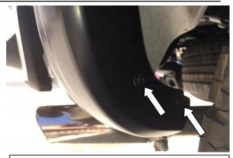
**STEP 15:** Place Fender Flare on the vehicle into the position of best fit. Note where the slots in Fender Flare align with the previously removed factory screws in the front and rear mud guards. Peel back 2 inches of the red tape liner on the fender flare extrusion at both ends, ensure liner is on the outside of part ref to step 18. Using #15 Torx head screwdriver re-install the upper and lower screws from the rear factory mud guard through the slots in the Fender Flare.
