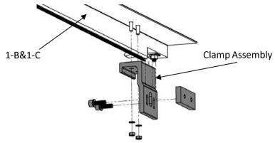
Step-2 Attach and Install the other set of Clamp Assembly (2-G) to the Side Rail (1-B&1-C), then tighten the nuts.
