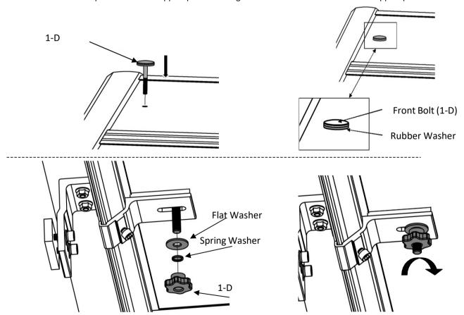
$\red{\%} \textbf{ATTENTION: Make sure the Flat Washer and Spring Washer are all placed on bolt before screw the plastic nut on.}$
