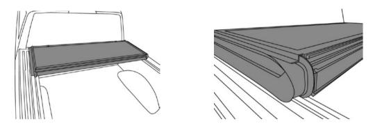
8. Adjust the front support plate(1-F) to correct position, insert the front bolt with rubber washer into the holes on the cover front panel and front support plate. Then tighten the hand nut under the front support plate.
