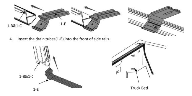
5. Unscrew and remove the aluminum block from the side rail. Insert the block into the truck bed Factory Track.
