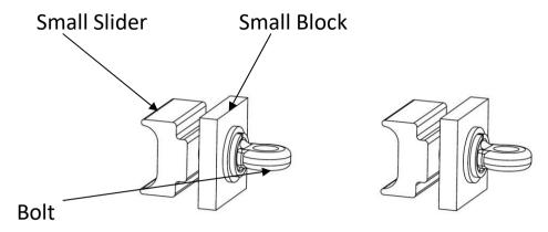
Insert the small slider into the Track Channel. Tighten the bolt. (Note: Make sure the small slider is installed nearby the Strap Safety Buckle position) There is a hole on the bottom of the bolt. Snap the safety buckle into the hole of the bolt.
