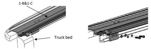
7. Place the bed cover on the front end of truck bed. Ensure the cover is even on all sides and sit firmly on side rails.
