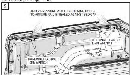
5. Once the mounting rails are in place, apply pressure while tightening the bolts to assure rails are sealed against the bed cap. (The use of a ratchet, 1/2" or 13MM socket or wrench for the front bolts and 10MM wrench for the rear bolts is recommended). The assistance of another person may be needed for this step to get the proper seal.
