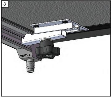
7 & 8. Assemble the four retainer clamps, slide each of them into the track on the underside of the tonneau, slide into position, but do not tighten at this time.
