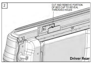
2. Locate the outlined section on the inside of the bed cap towards the tail light well at the rear of the bed. Cut and remove the outlined section of bed cap to reveal threaded holes. Repeat process for both Driver and Passenger side.
