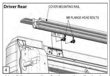
4. Install the rear portion of each mounting rail, using the M6 Flange head bolts and thread them into the pre-threaded holes located previously from the removed portion of the bed cap. Repeat process for opposite side. Leave bolts loose and proceed to step 5.
