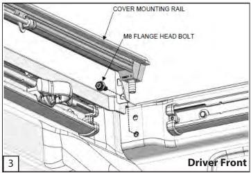
3. Using one of the M8 Flange head bolts, install the driver side mounting rail to the front bulkhead with using the lower hole in the flange on the front of the mounting rail and lower threaded hole on the bulkhead. Leave loose until rear mounting bolts are installed. Repeat process for passenger side.
