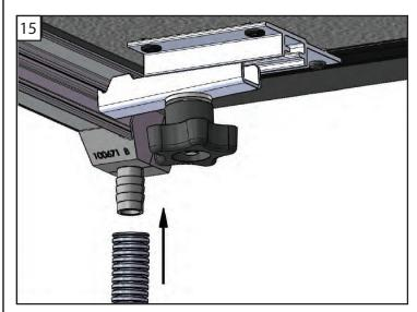
15. Attach the drain tubes to the fittings at the front of the bed rail and position the tubes to divert water out of the truck bed. This can be done by placing the tube behind a bed liner, through an existing hole in the bed, or by drilling a 5/8" hole in the bulkhead or bed floor.
