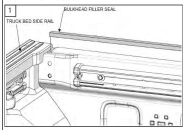
1. Install the bulkhead seal on top of the front bulkhead of the bed, centering the bulkhead seal front to back. Make sure to place the bulkhead seal, so that both ends set flush against the inside edge of the plastic bed rail caps, ( driver to passenger side ). Trim to fit.
