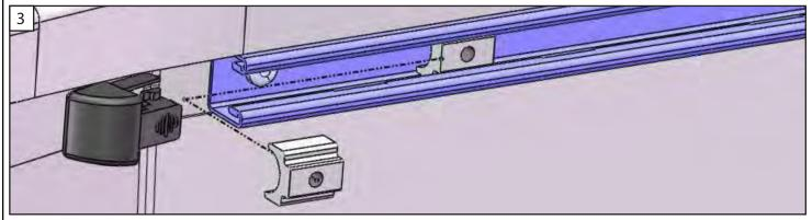
3. Slide the clamp assembly (3 per side) into the Utility rail, position one front, one center and one rear.
