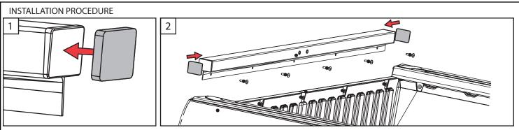
1 & 2. Using a T30 torx driver, remove the 5 fasteners securing the header rail to the bulkhead at the front of the bed. Adhere the gasket to the header rail end caps and reinstall the header rail.
