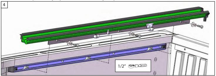
4 & 5. Using three (3) bolts per side attach both left and right side rails to the truck bed, Figure 2. The end of the mounting rail with the drain tube fitting will go towards the cab of the truck. Tighten the bolts using a 1/2" wrench or socket.
