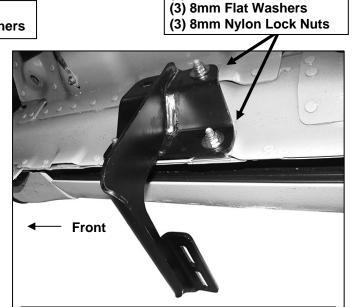
(Fig 4) passenger side front bracket installation
