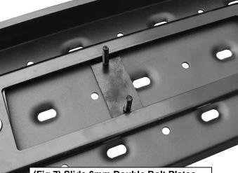
(Fig 7) Slide 6mm Double Bolt Plates into track on bottom of Step
