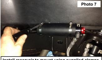
Install reservoir to mount using supplied clamps.
