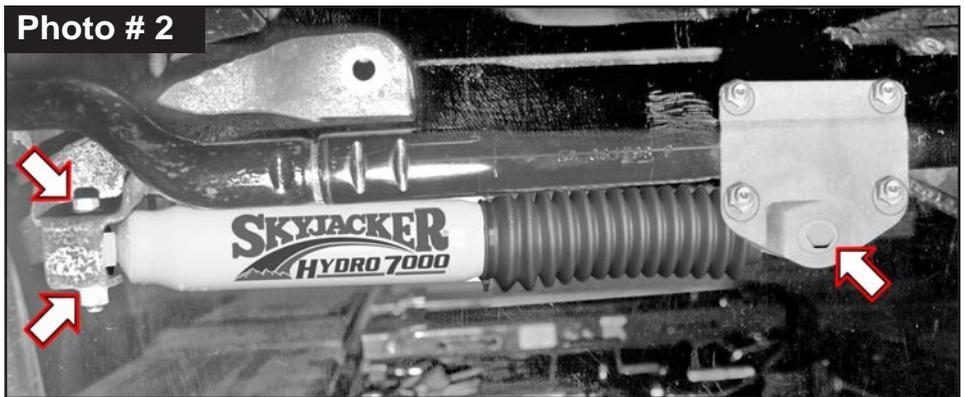
4. Next, extend stabilizer shaft end out & attach to driver side OEM tie rod mount.
