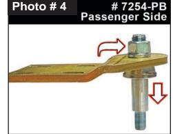
11. Extend each Skyjacker Tie Rod Bracket \ Shaft End out half way. **4-3/4"-5**".
