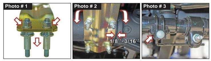
5. <u>Note</u>: Skyjacker Tie Rod Brackets Are Side Specific: Driver # 7218-DP & Passenger # 7254-PB.
