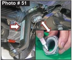
Attach Skyjacker Pitman Arm with OEM pitman arm nut using a 46mm socket\wrench. (Photo # 50) Torque to 350 ft-lbs. **Proceed to Step 40.**
