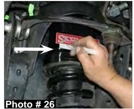
39. Remove the strut / spacer assemblies. Align the previously made marks & tighten the new strut spacers to the OEM strut assemblies using a 15mm socket. (See Photo # 27)
