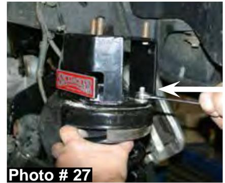
40. Install the strut / spacer assemblies by aligning the three upper strut mount studs with the OEM mounting locations using the supplied 10mm nuts & a 15mm socket. (See Photo # 28)
