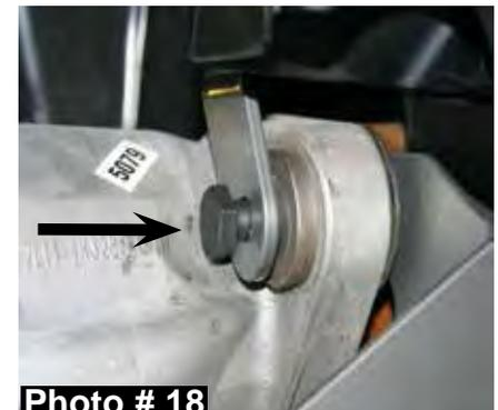
28. Install the two supplied 13/16" long crush sleeves, two 1/2" x 2" bolts, four 1/2" washers, & two 1/2" nuts in the two front holes of the passenger side OEM cross member bracket & new Skyjacker cross member using a 3/4" socket & wrench. **Do not tighten at this time.** (See Photo # 19)
