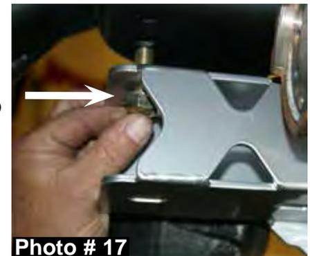
26. Install the supplied 14mm x 90mm bolt & 14mm nut in the lower mounting hole of the new Skyjacker driver side rear differential bracket & rear cross member using a 21mm socket & 22mm wrench. **Do not tighten at this time.** (See Photo # 18)
