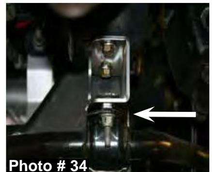
54. Connect the OEM sway bar end links to the OEM sway bar using the OEM hardware & a 18mm socket.
