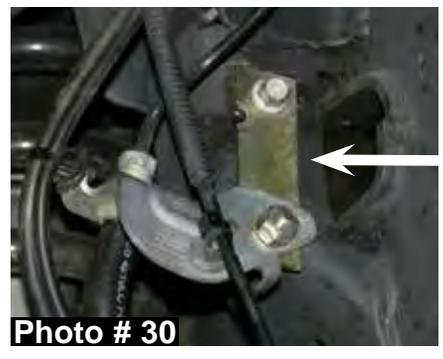
48. Disconnect the OEM front brake line brackets from the frame & install the new Skyjacker front brake line extension brackets using the OEM hardware & the supplied 1/4" x 1" bolts, nuts, & washers. (See Photo # 30)
