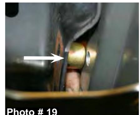
32. Tighten the 14mm x 90mm bolt, 14mm nut, & OEM bolt on the upper & lower mounting locations of the new Skyjacker driver side rear differential bracket & rear cross member using a 21mm socket & 22mm wrench.
