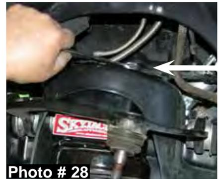
42. Install the OEM 4WD actuators using the OEM hardware & a 8mm socket. **Note:** Make sure that the OEM hose connections are pointing upward. (See Photo # 6)
