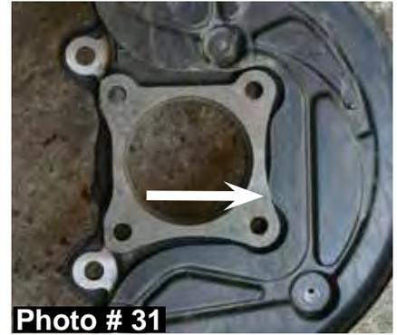
50. Install the OEM brake rotors, brake line brackets, & brake caliper assemblies using the OEM hardware. **Note:** If the OEM brake caliper mounting hardware is 14mm, place the supplied (two per side) reducer bushings (Part # 1416-BSG) in the OEM brake caliper mounting locations of the new Skyjacker steering knuckles before installing the OEM 14mm hardware. (See Photo # 32)
