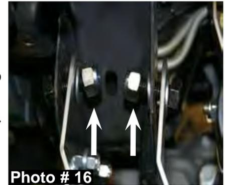
25. Install the two supplied 1/2" x 1 1/2" bolts, four 1/2" washers, & two 1/2" nuts in the two holes of the new Skyjacker intergrated sway bar lowering bracket using a 3/4" socket & wrench. **Do not tighten at this time.** (See Photo # 17)
