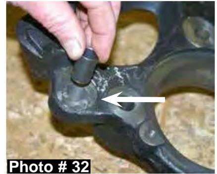
51. Install the OEM outer tie rod ends to the new Skyjacker steering knuckles using the OEM hardware & a 21mm socket. (See Photo # 1)
