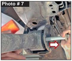
Disconnect OEM rear LCA from front OEM frame mount using a 24mm socket\wrench. (Photo # 7) Remove OEM tab bolt & lock nut. Remove OEM rear LCA.
