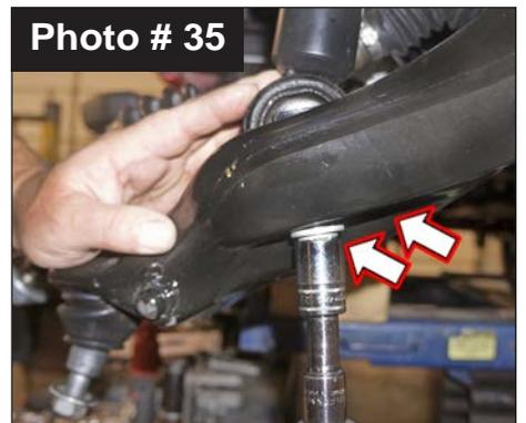
36. Guide CV axle through OEM knuckle \ hub assembly and connect lower control arm ball joint to knuckle. Install factory nut using a 21mm wrench.
