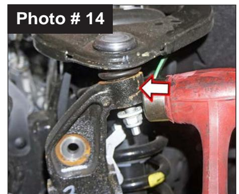
16. Loosen, but do not remove OEM lower control arm ball joint nut from OEM knuckle using a 21mm wrench. (See Photo # 15) To unseat ball joint taper, strike ball joint boss of knuckle to dislodge.
