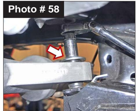
64. Once all differential mounting brackets have been installed, remove jack then tighten and torque all hardware at this time. Torque passenger side differential bracket supplied 10mm bolt to 45 ft.-lbs. using a 13mm socket \ wrench. (See Photo # 58)
