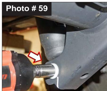
5. Remove OEM u-bolts using a 21mm socket \ wrench. Discard u-bolts and hardware. Retain lower OEM u-bolt plate. (See Photo # 60)
