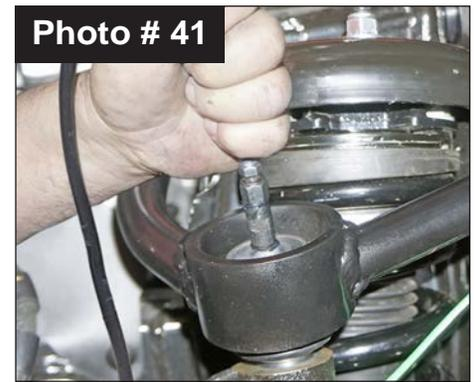
44. Connect OEM sway bar end link to OEM knuckle using 18mm socket \ wrench. (See Photo # 9)
