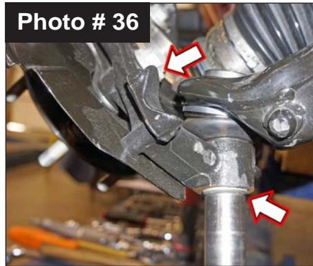
37. Connect upper OEM ball joint nut to OEM knuckle with supplied Castle Nut and Cotter Pin using a 18mm wrench.
