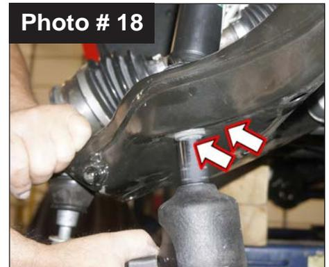
18. Disconnect two (2) OEM lower strut mounting nuts from lower control arm mount using a 18mm socket \ wrench. (See Photo # 18)
