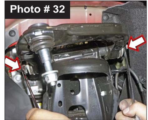
32. Install Skyjacker Upper Control Arm to appropriate side of vehicle using OEM hardware, an 18mm and a 21mm socket \ wrench. (See Photo # 33)
