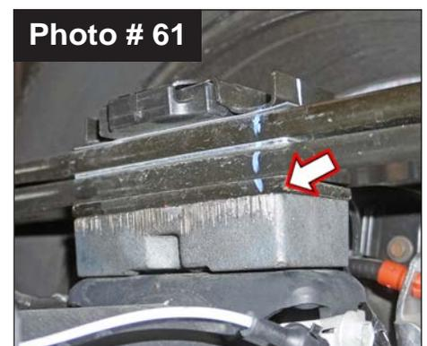
9. Install Skyjacker 9/16" U-Bolts over OEM top plate\leaf springs down into OEM u-bolt plate. Install supplied 9/16" Nylon Insert Nuts using a 7/8" socket\wrench. Torque u-bolts evenly using an 'X' crisscross tightening sequence. Torque to 90 ft.-lbs. (See Photo # 62)
