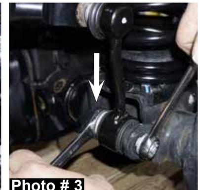
6. Disconnect the OEM front track bar from the frame using a 21mm socket / wrench. (See Photo # 4)
