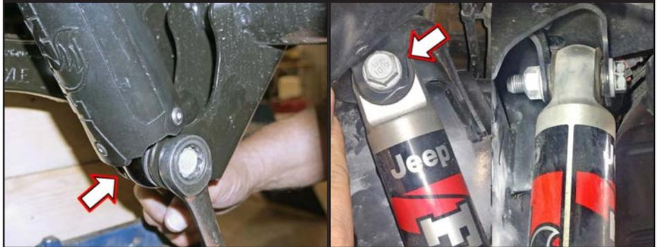
6. Assemble Skyjacker # GULR24-SX-L Rear Upper Flex Link with # RE114-640R Right Hand 1-1/4" Rod End & # 114RFTJN Jam Nut. (See Photo # 27)
