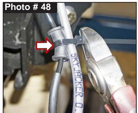
23. Attach OEM ABS line at rubber grommets to Skyjacker brake lines with supplied plastic ties. Trim with Diagonal Cutting Pliers. (See Photo # 48)
