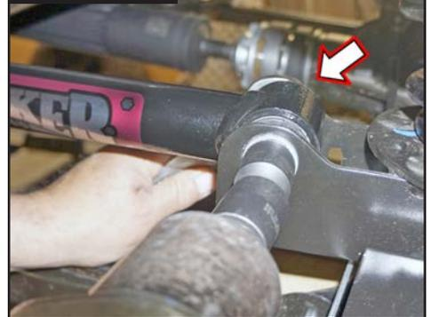
One at a time, install Skyjacker # GULR24-SX-L Rear UCA with OEM hardware using a 21mm & a 24mm socket \ wrench. (See Photo # 29)
