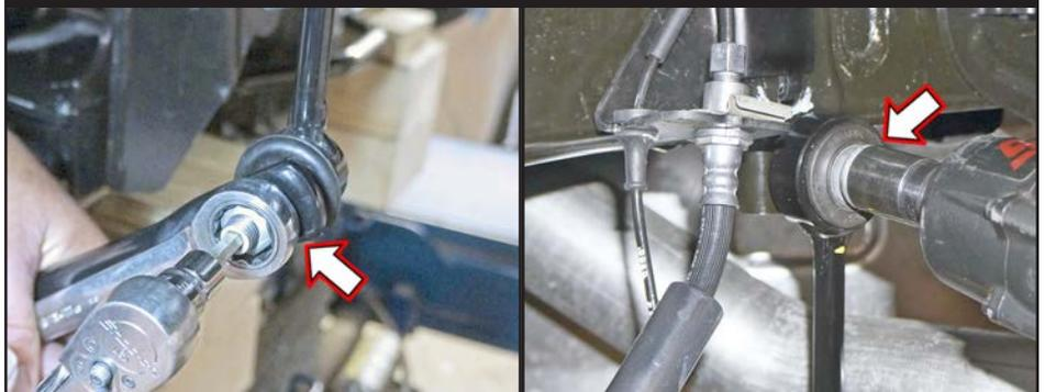
4. Disconnect OEM rear track bar from rear axle mount using a 21mm socket \ wrench. (See Photo # 25) **Tech Note:** It may be necessary to raise \ lower axle to take pressure off track bar bolt. Retain OEM hardware.
