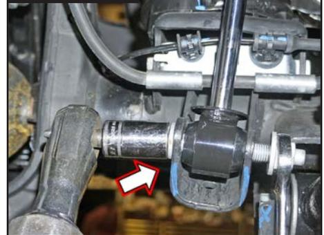
24. **Tech Note:** ADX Remote Reservoir are to be mounted with cylinder body up & remote reservoir toward rear for proper clearance (opposite side of coil spring mount).
