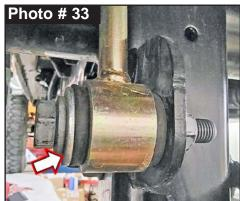
Attach lower end link with OEM hardware with large washer to bushing side of end link using a 18mm socket\wrench. (See Photo # 33) Secure, but **Do Not Completely Tighten** at this time.
