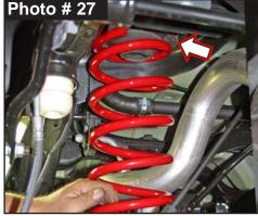
Be sure coil spring is seated properly at lower axle mount by rotating the coil until the pigtail hits the spring stop. **Note:** Be sure OEM upper coil spring isolator is properly aligned with coil & upper coil spring mount. (See Photo # 27) Raise rear axle to load Skyjacker rear coil springs.
