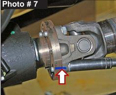
drive shaft to ensure the drive shaft does not bind when installing taller springs. Mark the location of OEM front drive shaft\flange at axle & disconnect using a 15mm socket\wrench. (See Photo # 7)
