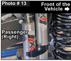
Install Skyjacker ADX front shock at upper shock tower mount with supplied stud bushings, cup washers & nut using a 14mm socket\wrench.
