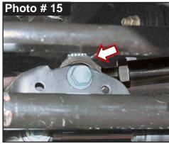
Completely Tighten at this time.
