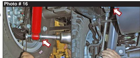
Remove upper mount to sway bar using a 19mm socket\wrench.
