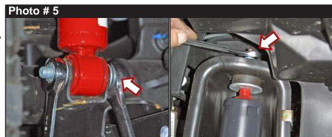
Disconnect OEM front brake line bracket using a 10mm socket\wrench.
