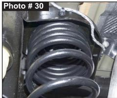
Raise the rear differential in order to load the Skyjacker rear coil springs.
