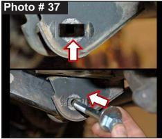
3. Connect OEM front lower control arm to modified OEM front axle mount using Skyjacker eccentric cam bolt, eccentric washer, nut, a 21mm socket\wrench & a 24mm socket\wrench. (See Photo # 38)
