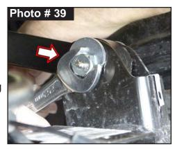
5. With vehicle on ground & weight of vehicle on tires\wheels, tighten front & rear eccentric cam bolts using a 21mm socket\wrench & 24mm socket\wrench.
