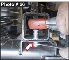
Check fit Skyjacker # JLRTBU-B Rear Track Bar Upper Bracket over OEM rear upper track bar mount on frame. The double hole side of Skyjacker track bar bracket towards outside of vehicle. (See Photo # 28)
