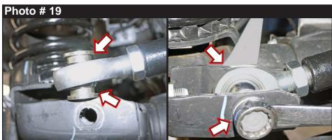
Fully tighten all OEM hardware at upper frame mount & axle mount. Fully tighten jam nut of Skyjacker adjustable front track bar using a 1-1/8" wrench.
