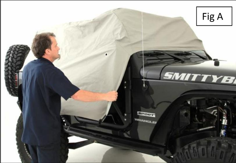
**Step 2:** Locate the side straps and attach below the door. Tighten straps slightly to keep them hooked on the vehicle. Once all straps are in place, tighten down evenly to secure the cover to the vehicle. Some nerf bars may prohibit the strap to be attached to the pinch weld. You may loop strap around body mount bolt and then attach to body mount cup or other location on the body tub. Fig B+C. Pull straps snug, but Do not over tighten straps, damage to cover and/or vehicle may occur.
