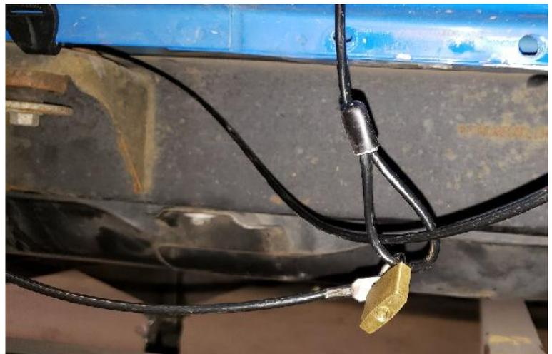
Short cable only hooks to one side of vehicle around body mount. Lock junction placed away from painted body to avoid damage.
