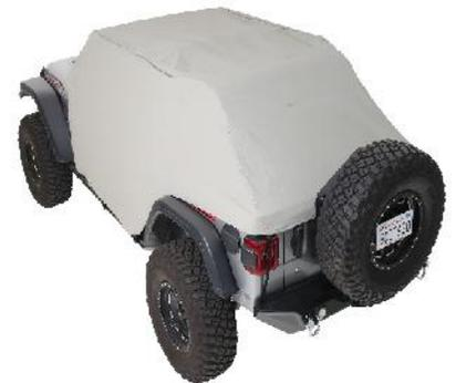
**JL-** Secure the rear corner straps to the bottom of the body and or accessory in the same proximity. Note: you may need to slide strap behind the bumper starting at the end of the bumper. (Fig 1,2)
