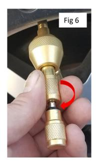
6. Remove air down gauge by turning valve stem adapter counter clockwise until it is removed from the valve stem. Always replace valve stem cap to prevent dirt and debris from damaging valve core. Fig 6
