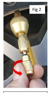
2. Push on the valve core remover and turn counterclockwise to remove valve core. Fig 2
