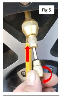
5. Once desired air pressure is achieved , keep slide valve pushed in and reinstall valve core by pushing in on the valve core remover and turn clockwise to install valve core. Tighten until snug. DO NOT over tighten. Fig 5
