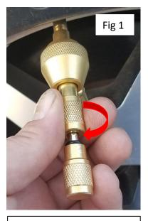
1. Thread valve stem adapter onto valve stem till snug. <u>NOTE:</u> If you push in on the valve core remover firmly, the gauge will read current tire pressure. This feature works with most valve stems. Fig 1.
