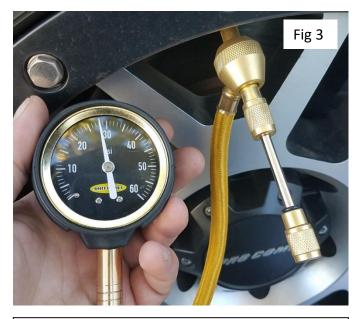
3. When valve core is unthreaded, air pressure from the tire will push the valve core remover out and the gauge will read the tire pressure. Fig 3
