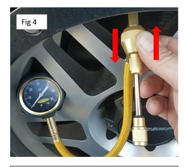
4. Pull out on the slide valve to release pressure. Push slide valve in to stop bleeding pressure and to read tire pressure. Fig 4
