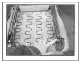
Step 3: Place the sliders you just removed onto the new seat. Re-use the spacers (if separate)
