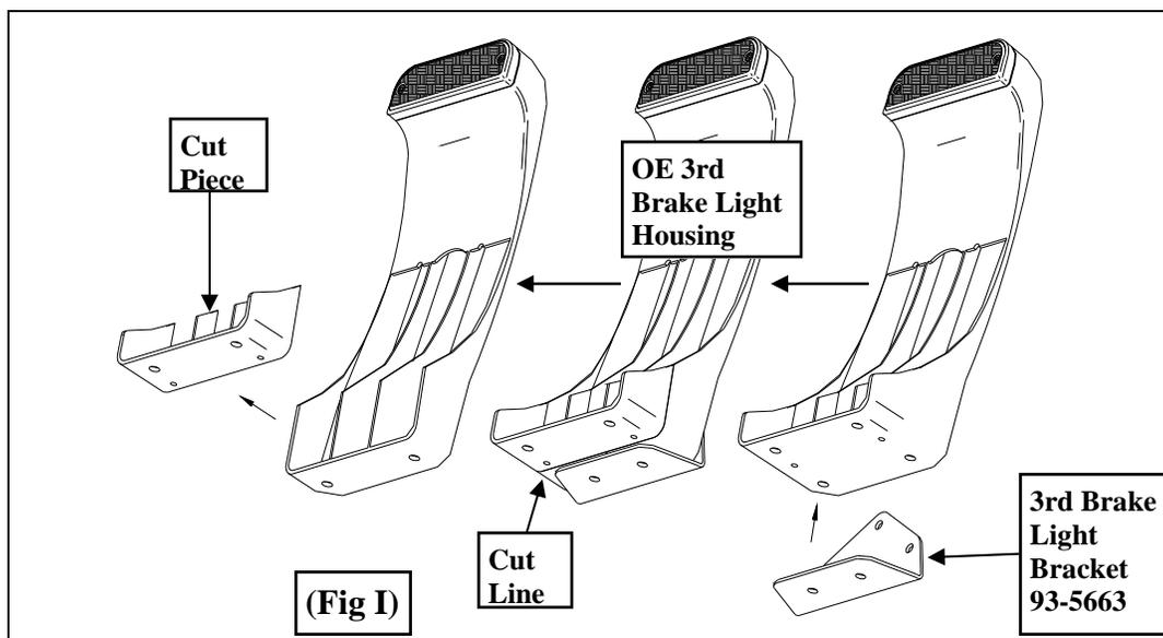
**Step 3:** Once the OE 3rd brake light plastic housing has been properly trimmed, place it flush against the back 3rd brake light bracket (93-5663). Use the (3) holes in the bracket as a
