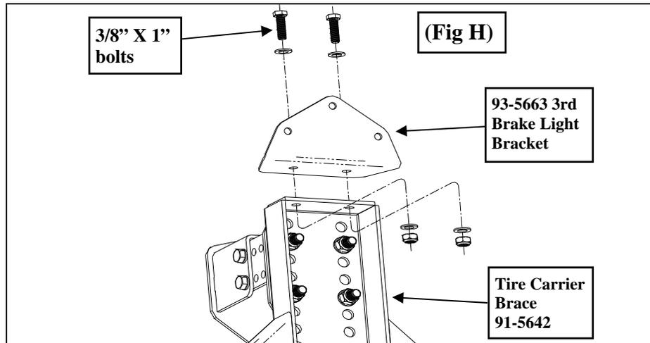
**Step 2:** Place the OE 3rd brake light plastic housing flush against the back of the 3rd brake light bracket (93-5663). Using the bracket as a guide, scribe a line across the bottom of the plastic light housing. Trim the plastic housing along the scribed line. (Fig. I)
