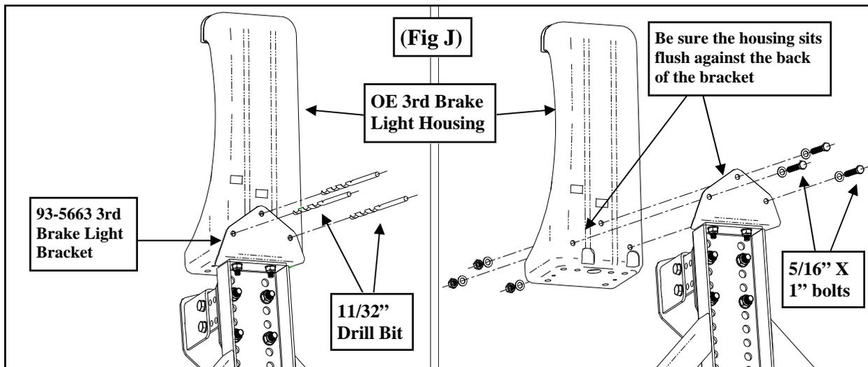
**Step 5:** Reconnect the 3rd brake light wiring harness.
