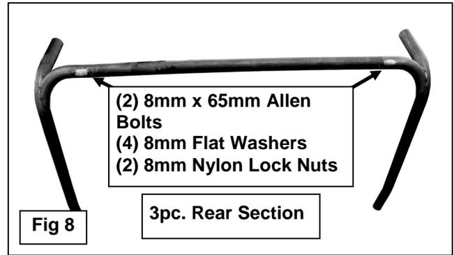
9. With assistance, attach the assembled rear top section of the Roof Rack to the already inserted Side Rails. **NOTE:** Be careful not to damage the vehicle when attaching the top section. Use the included (2) 8mm x 65mm Allen Bolts, (4) 8mm Flat Washers and (2) 8mm Nylon Lock Nuts to attach the Rear Top Legs to the Side Rails, (**Figure 9 & 10**).
