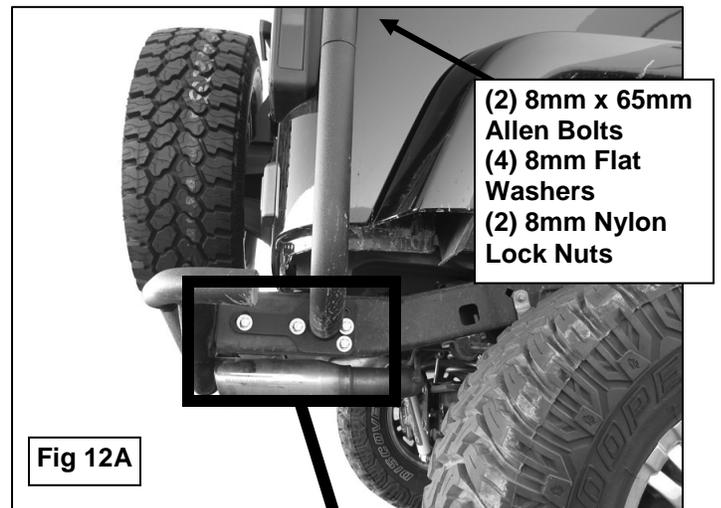
**Note:** Installation shown with aftermarket bumper. Use the included Double Nut Plate, **(N)**, inside the rectangular frame tube as required for installation on vehicles without rear bumper or aftermarket bumpers that are not threaded for mounting bolts. Also use the following hardware included with this kit as needed:
