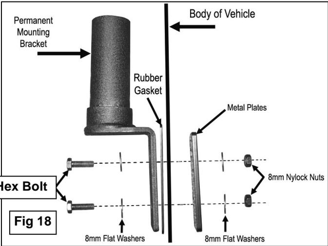
24. Insert (2) 8mm x 35mm Hex Head Bolts with (2) 8mm Flat Washers through the Short Bottom Brackets and body. Access the hardware through the opening for the taillight and position the 2-hole Metal Plates over the already inserted 8mm Hex Bolts, **(Figure 19)**.
