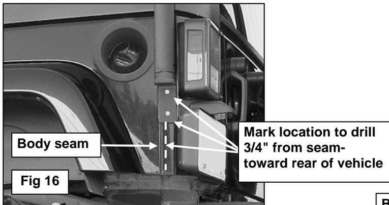
20. Once you have marked the drill locations on both sides of the vehicle, remove the rear assembly of the Roof Rack and set it aside. **NOTE:** Do not remove the Short Bottom Brackets from the Rear Legs.
