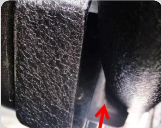
**Note:** It is recommended that you position your tire against the Tire Carrier frame so that when you tighten the lug nuts it pushes the tire against the Carrier. This prevents the sidewall from flexing and creating a vibration.
