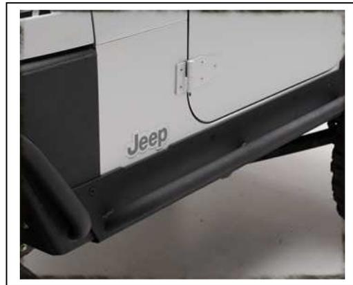
**Step 1:** Take off and remove any existing flares or rocker guards that you may have on your vehicle. (Fig A) Make sure to clean the side of the vehicle before installing the guards.
