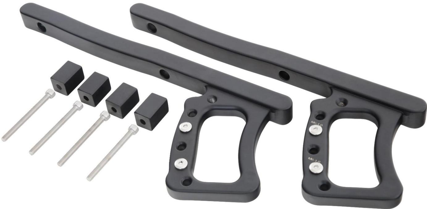
**Note:** The handles feature M6-1.0 threaded holes for mounting of additional custom accessories (not available from Smittybilt). Do not over tighten bolts.
