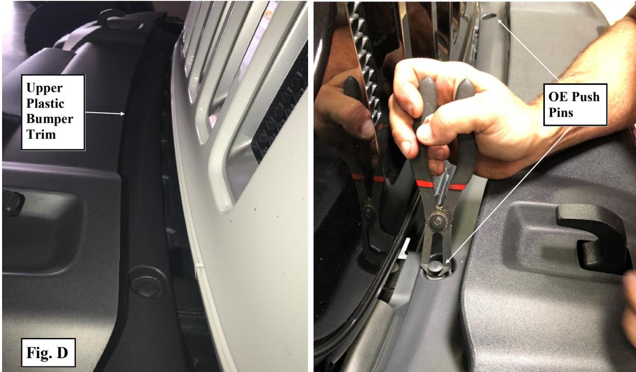
**Step 6:** Carefully remove the OE front bumper from the vehicle.
