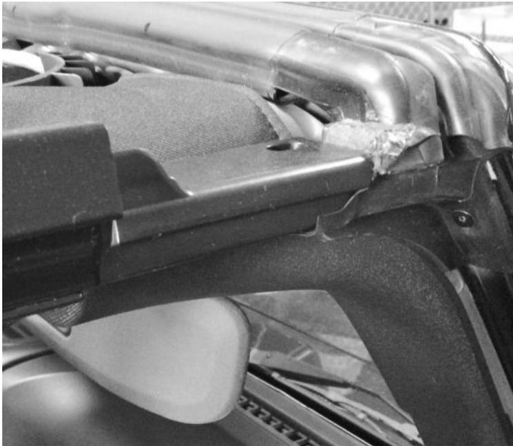
**NOTE:** Pay close attention to the rubber gasket at the top of the windshield and how the front section inserts into it. The picture to the left shows how it should fit.
