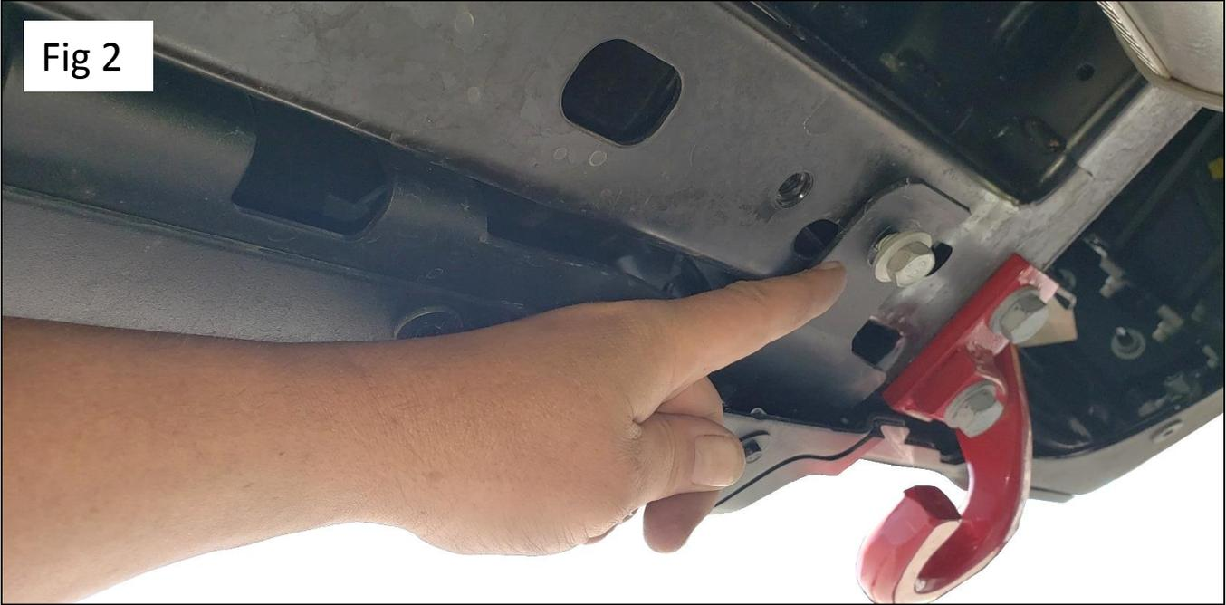
**Step 3:** If equipped, remove the two bolts and nut plate from rear cross member. It will not be reused. Fig 3.
