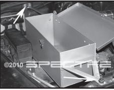
Step 5 Install the box and install the factory bolts for the core support and firewall. These two bolts will be threaded on just enough leaving enough play allowing yourself to line up the holes in box with the free standing spacers.
