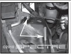
Set the two spacers on the inner fender. See picture for locations.
