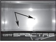
Step 6 Install the supplied hardware the bolts facing downward. Once set in location, install the washer and nut on the underside of the fender and securely fasten in place.
