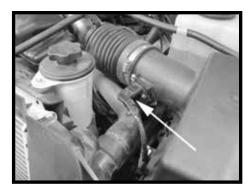
Step 2 Slide the red clip back then disconnect the electrical connector at the Mass Air Flow Sensor (MAFS). Unclip the wiring harness from the air box base.
