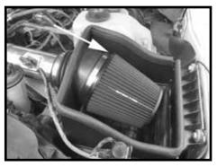
Step 16 Install the supplied air filter and clamp and tighten the clamp that secures the air filter. If needed, rotate the air filter/velocity stack adapter assembly for the maximum clearance as shown.
