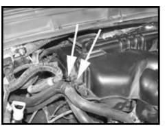
Step 4 Unclip the engine coolant line and the wiring harness that is connected to the plenum.
