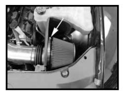
Step 15 Install the filter on the velocity stack adapter and fasten it securely. If required rotate the velocity adapter so the filter will fit without any fitment issues.
