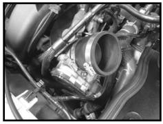
Step 11 Install the provided coupler reducer onto the throttle body and secure with provided hose clamp.
