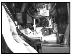
Step 10 Remove the bolt shown in the picture then lift up and remove the intake silencer from the vehicle.
