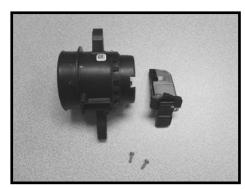
Step 22 Remove the 2 screws securing the mass air sensor then remove the mass air sensor from stock housing.
