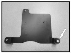
Step 13 Install the provided rubber mount stud onto the heat shield base as shown using the provided hardware.
