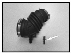
Step 20 Remove the EVAP fitting form the intake hose
