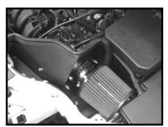
Step 36 Install the 30" long section of edge trim onto the fresh air plate and heat shield as shown. Some trimming of the edge trim will be necessary.
