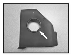
Step 25 Install the supplied rubber trim molding into the heat shield side.
