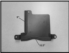
Step 15 Install the 9" and 10.5" pieces of edge trim onto the heat shield base as shown.
