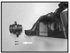
Step 21 Remove the 2 bolts securing the mass air sensor housing to the air box and separate the mass air housing from the air box.
