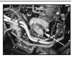
Step 6 Install the throttle body adapter ring onto the throttle body.
