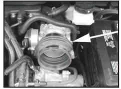
Step 12 Install the flex coupler on the throttle body and secure the boot in place. Install a second clamp but do not tighten at this time.
