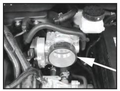
Step 11 Install the throttle body adapter ring onto the throttle body.
