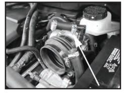
Step 15 Install the hose and secure it with the provided clamp. Install a second clamp but do not tighten at this time.
