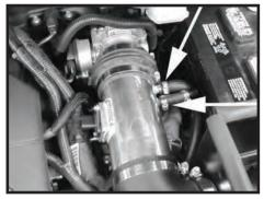
Step 17 Connect the two vent lines to the intake tube and fasten the clamps securely in place.
