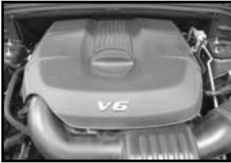
Step 2 Start by removing the engine cover that is attached by small ball and socket joints.
