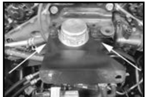
Step 10 Install the provided intake tube bracket onto the air injection pump mounting studs, reinstall the air injection pump and secure it with the nuts removed in Step 9.
