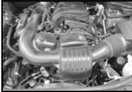
Step 6 Remove the factory air intake tube for the vehicle.
