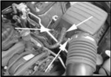
Step 5 Loosen the clamp at the throttle body and disconnect the breather line from the air box lid. On the back side of the air box unclip the hose from the air box lid.
