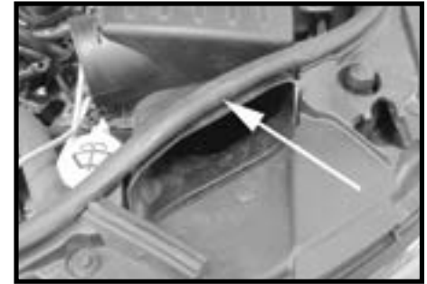
Step 7 Unclip the factory edge trim from the scoop.
