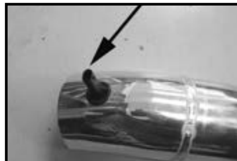
Step 12 Install the supplied grommet into the intake tube then install IAT sensor into the grommet.
