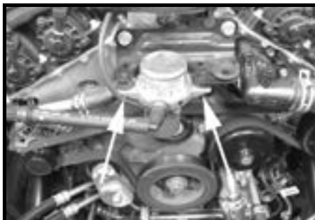
Step 9 Remove the two nuts that secure the air injection pump.
