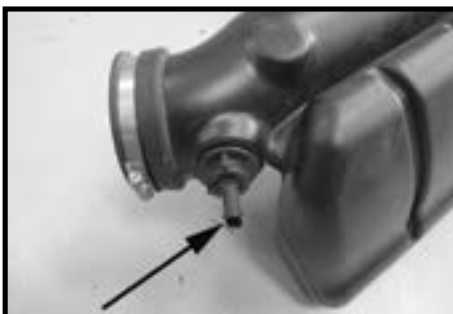
Step 11 Turn the IAT sensor counterclockwise and remove it from the factory intake tube. Remove the O-ring from the sensor.
