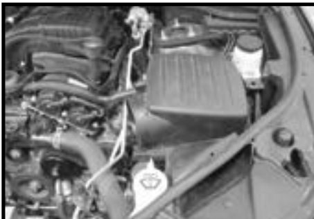
Step 8 Remove the air box by pulling up and out firmly.
