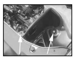
Step 11 Install the heat shield into the vehicle. Reuse the factory bolt from Step 4 and use the supplied hardware for the rubber insert.
