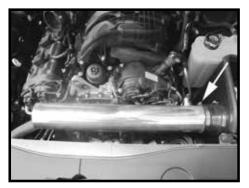
Step 14 Install the intake tube as shown making sure the small vent tube closest to the heat shield.
