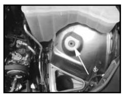
Step 10 Install the rubber insert in the hole located on the inner fender.
