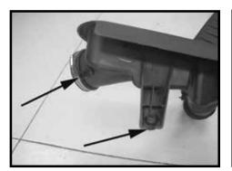
Step 5 Turn the IAT sensor counterclockwise and remove it from the factory intake tube. Remove the O-ring from the sensor. Remove the intake plenum mount grommet from the intake plenum.
