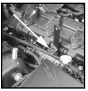
Step 12 Install the bracket onto the mounting stud as shown.
