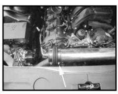
Step 15 Install the flex coupler onto the end of the tube and fasten it securely, leave the other clamp loose at this time.
