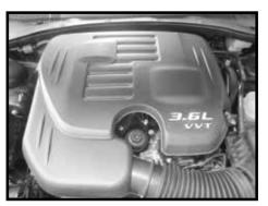
Step 2 Remove the engine cover.
