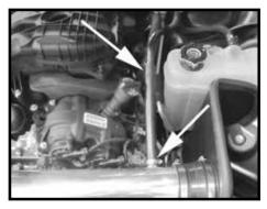
Step 18 Connect the breather hose to the existing plastic vent line, then to intake tube. Once in desired position fasten securely in place. NOTE: On later model vehicles with the CCV connection near the throttle body, it will be necessary to use the provided quick connect fitting and longer CCV hose.
