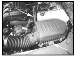
Step 4 Remove the breather hose from the plastic vent line. Remove the screw holding the factory air box in place and set it aside, this will be used in a later step. Remove the factory air intake system from the vehicle.
