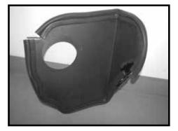
Step 8 Dress the heat shield with edge trim as shown. This may require trimming to the correct length.
