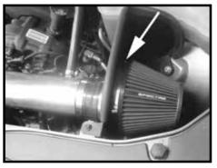
Step 19 Install the filter on the velocity stack adapter and fasten it securely. If required rotate the velocity adapter so the filter will fit without any fitment issues.
