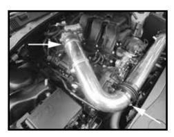
Step 16 Install the second intake tube into the throttle body coupler first then into the flex coupler. Once in desired position fasten securely in place.
