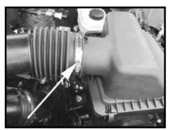
Step 2 Loosen the clamp from the intake tube to the air box lid.
