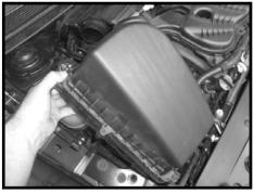
Step 5 Lift up to release the mounting studs holding the air box and lift the air box out of the vehicle.
