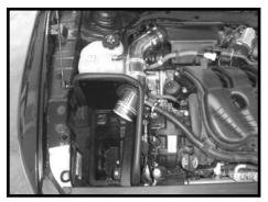
Step 8 Install the intake tube into the hole in the heat shield. Install the intake assembly into the vehicle as shown while making sure the plastic mounts capture into the locating grommets.
