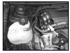
Step 7 Install the provided coupler on to the vehicle as shown.
