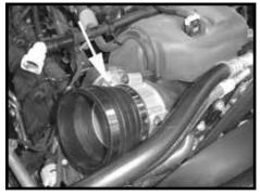
Step 10 Install the provided reducer coupler onto the throttle body as shown.
