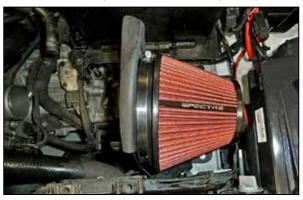
13. Install the filter assembly into the heat shield and secure with the rear mounting bolt provided only at this time.
