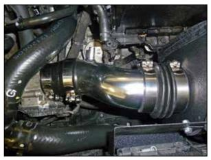
17. Install the intake tube into the coupler hose at the throttle body fully then into the coupler hose at the filter adapter, adjust the tube for proper fit and then secure with the provided hose clamps.
