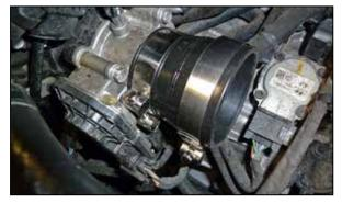
15. Install the provided silicone step coupler onto the throttle body and secure with the provided hose clamp.
