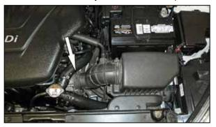
2. Loosen the hose clamp securing the intake tube to the throttle body.
