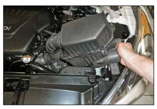
5. Remove the air box assembly from the vehicle.
