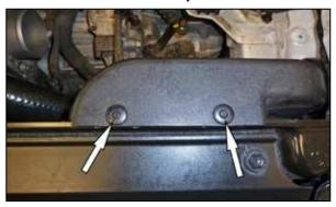
6. Push in the center of the fresh air duct retaining clips and then remove the clips.
