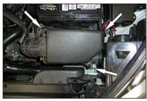
4. Remove the three bolts securing the factory air box assembly onto the inner fender.
