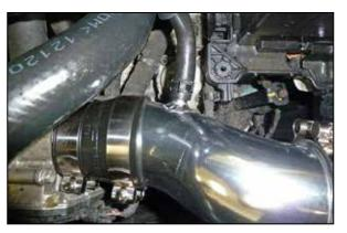
18. Reroute the crank case vent line under the fuel line and then install it onto the crank case vent fitting on the intake tube.
