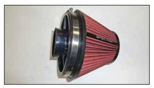
12. Install the filter adapter into the SPECTRE® air filter and secure with the provided hose clamp.
