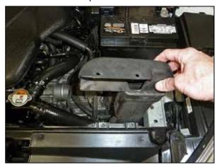
7. Remove the fresh air intake duct.
