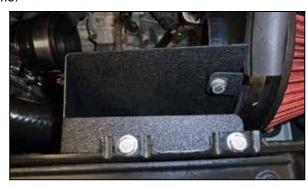
14. Install the fresh air intake scoop and secure to the core support and heat shield/filter adapter with the provided hardware.
