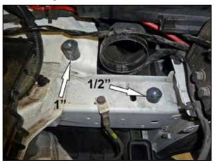
10. Install the 1" rubber mounted stud into the rear factory air box mounting location as shown. Install the ½" rubber mounted stud into the front factory air box mounting location as shown.
