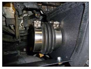
16. Install the provided flex coupler onto the filter adapter and secure with the provided hose clamp.
