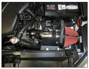
19. Make sure that all clamps and hardware are fully tightened. Reconnect the battery cable, start the vehicle and let it warm up. Shut off and inspect the installation once more for any loose clamps, wires, or hardware. Test drive & enjoy! Your installation is now complete. Periodically check all clamps and brackets.
