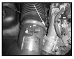
Step 3 Using a 5/16" nut driver (or flat blade screwdriver), loosen the clamp where the intake tube connects to the airbox.
