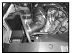
Step 11 Install the intake tube into the vehicle. Once the tube is roughly in place, install the velocity stack adaptor through the heatshield and onto the coupler. Once the tube is in desired location securely fasten the tube in place.
