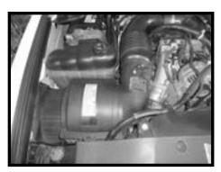
Step 4 Lift the stock air box assembly up and out of the engine bay assembly by pulling up and out firmly making sure to leave the stock intake tube in the vehicle.
