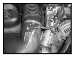
Step 2 Disconnect the Mass Air Flow Sensor (MAFS) electrical connector.
