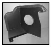
Step 8 Assemble the heat shield with the tabs placed on the outside of heat shield. Install bulb seal around edges of heat shield as shown.
