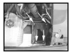
Step 4 Remove the four bolts (shown) and remove the factory air box tray from the vehicle.
