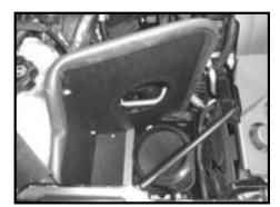
Step 12 Place the filter into the hole in the inner fender to be installed in later step.
