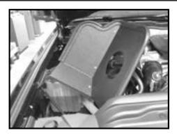
Step 10 Install the heat shield into the vehicle at an angle as shown.
