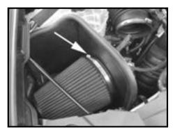
Step 14 Install the supplied air filter and clamp and tighten the clamp that secures the air filter.
