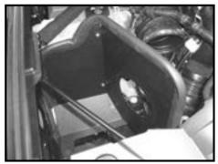
Step 11 Install the heat shield into the truck as shown by reusing three of the bolts removed in Step 4.
