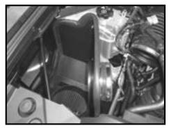
Step 13 Place the velocity stack adapter in the heat shield and install the supplied coupler making sure the coupler is pushed completely against the heat shield. Once the adapter and coupler are tight against the heat shield, tighten the clamp.
