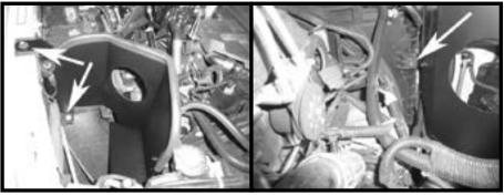
Step 10 Install the heat shield into the vehicle making sure the plastic air box mount goes into the factory grommet. Then secure the heat shield using the factory hardware removed in Step 9. Make sure the tab is placed on the outside of the radiator shroud for proper fitment.
