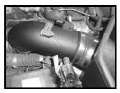
Step 13 Install the intake tube into the vehicle, position it as shown and once tube is in desired location fasten securely.
