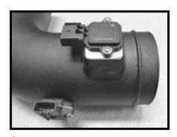
Step 12 Using the supplied screws, install the IAT and MAFS onto the tube.
