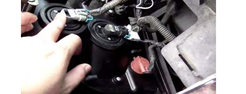
When installing the Headlight, insert from inside where the side bracket is showing, as shown in the picture
