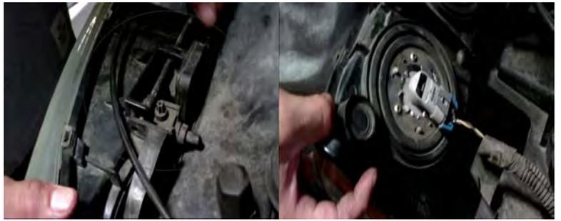
Transfer the bulb from the factory headlight to the new headlights. The top is Low beam, the bottom is high beam. Once you put the bulbs on, return to the truck and insert the turn signal, daytime running lights, and parking lights onto the socket.
