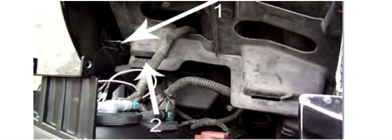
Insert the new clips on the grille, the longer clips is on top and the short one is on the bottom.
