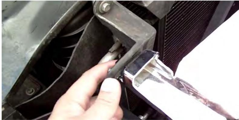
Pull the piece off from the Cover and insert it onto the grille as shown on the picture.
