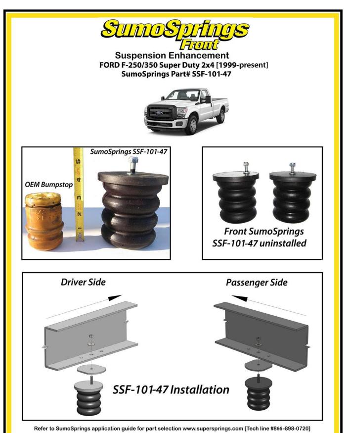
SumoSprings enhance load carrying capability, handling & towing. Never exceed vehicle manufacturer's GVWR rating.
