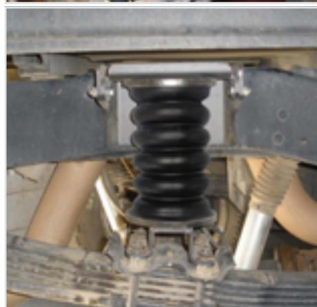
**ALTERNATE BOTTOM BRACKET ASSEMBLY (NOT TYPICALLY NEEDED)**
