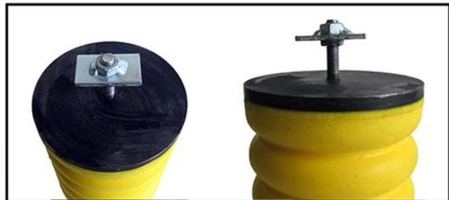
Insert plate into sideways slot at rear.
